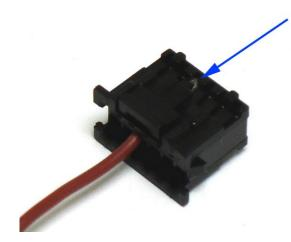
The terminal should be visible looking from above/ below the connector.
